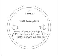
2 Fix the mounting base to the installation position according to the holes on the mounting template.
