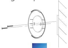
3 Line up and wedge the lower edge of the camera base with the mounting base and then push the camera to the mounting base to secure it.
