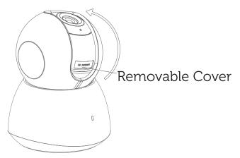
2 Open the cover to expose the memory card slot, and insert the memory card.
